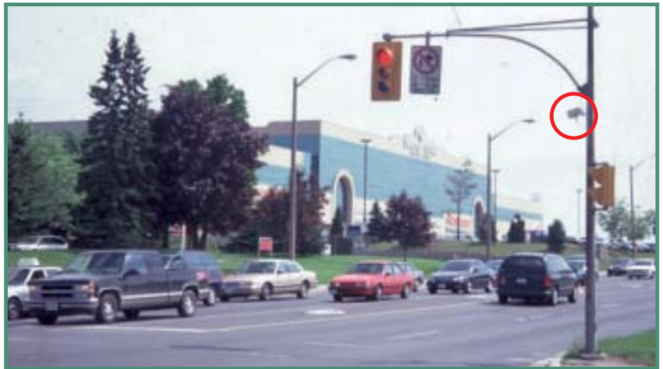
Actuated Signal Control
